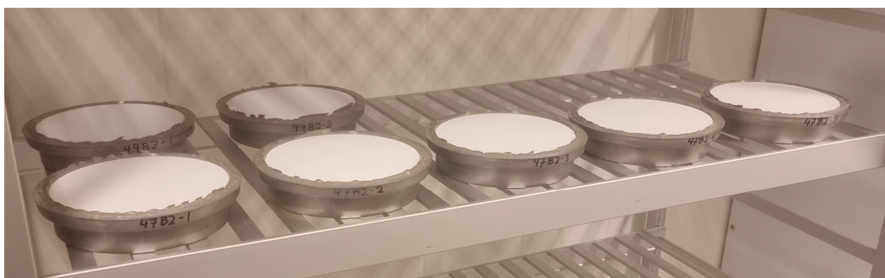
Figure 2. Samples of painted gypsum board, stored on shelves in a controlled climate chamber.
