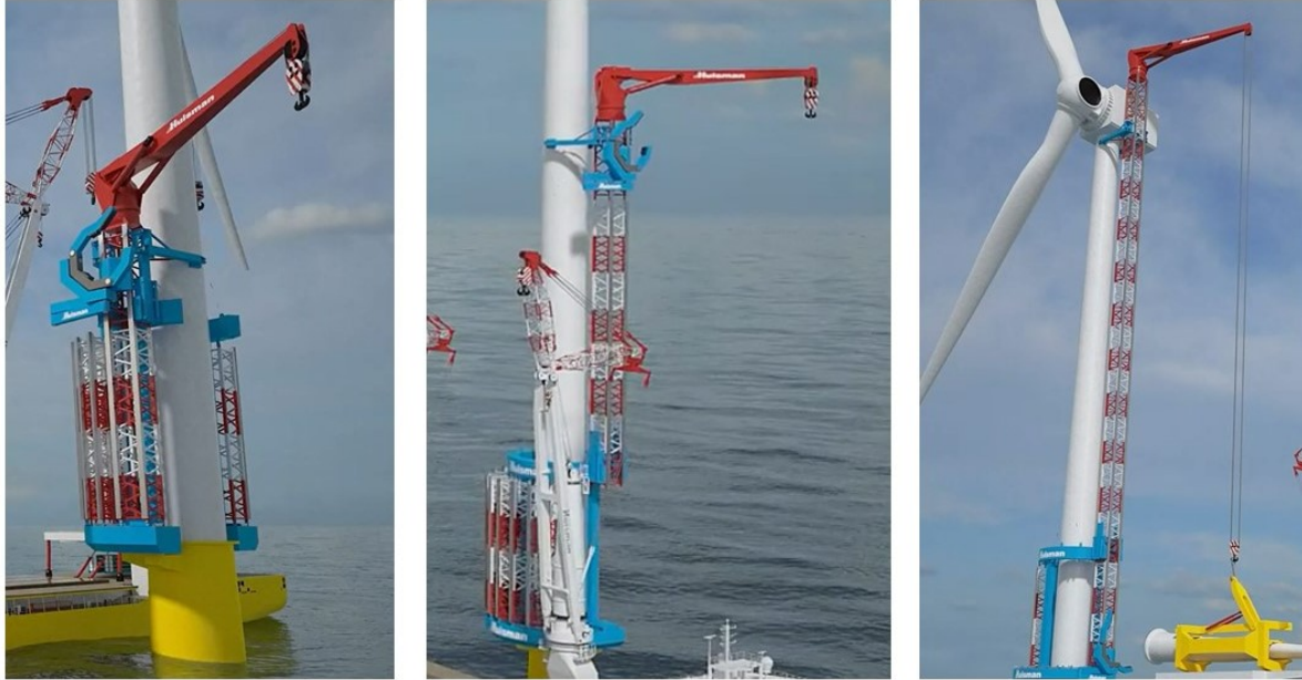
Figure 4.2: The climbing sequence of the OSCC, in which it can jack itself up starting from its compressed mode, to its extended mode
