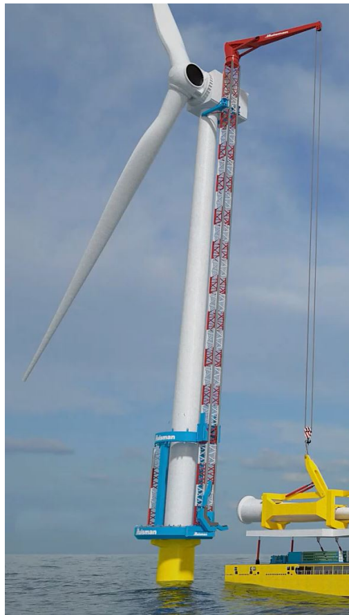
Figure 1.1: The Offshore Self-Climbing Crane that will be used as a case study in this thesis
