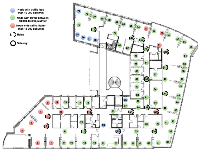
Fig. 2. The sensors, relays, and gateway in the test network.
