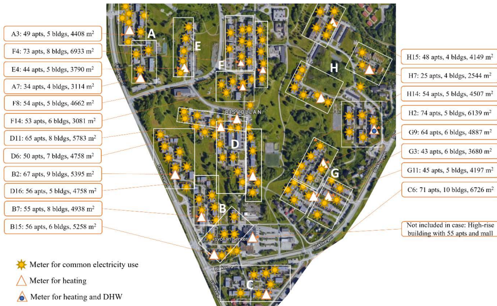
Figure 3 Case study area, with metering structure for common electricity and heating meters (Map: google maps).
