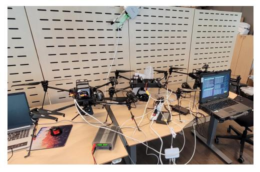
Figure 6.2: Ground testing arrangement with three Flamingo drones and one GCS at the laptop to the right
