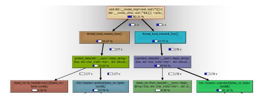
Figure 5.8: Callgraph for the transmit and receive functions
