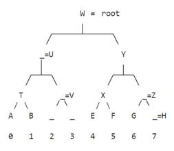
Figure 2.2: Example of a ratchet tree. Nodes represented by underscore are blank. The leaf nodes A, B, E, F, and G represent the group members. [2]
