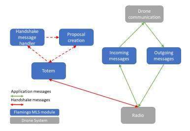
Figure 4.2: Technical overview of Flamingo MLS. All solid lines use UDP, while dotted lines represent communication through memory objects.
