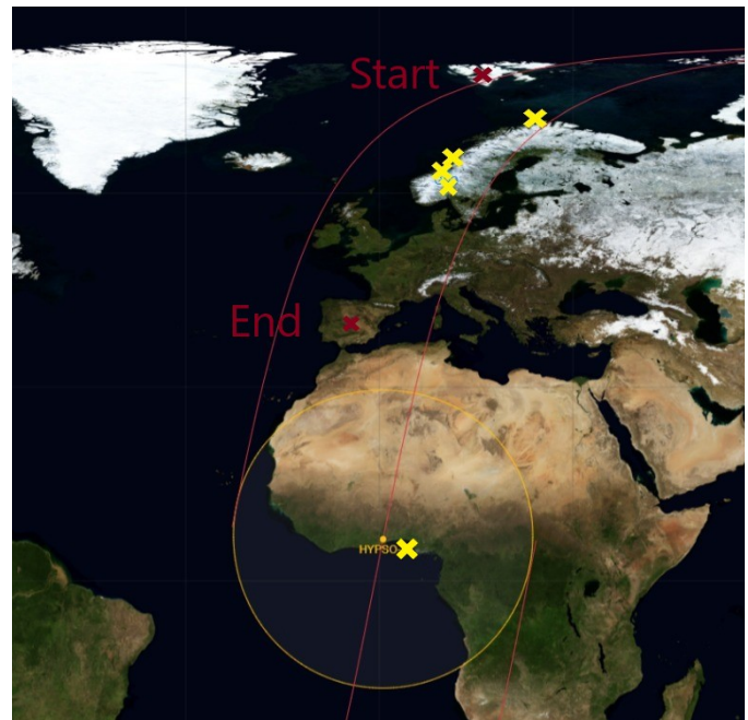
Fig. 5. Map showing the position and ground track of HYPSONO-1 as of March 14, 2023. A dark yellow circle marks the satellite, and the satellite ground track is marked in red. The initial target, Svalbard, and the final target, KSAT Spain, are marked by dark red crosses. The other targets are marked with yellow crosses following the satellite's path, going from North to South. The satellite is close to the 6th target in the figure, the Nigerian coastline.
