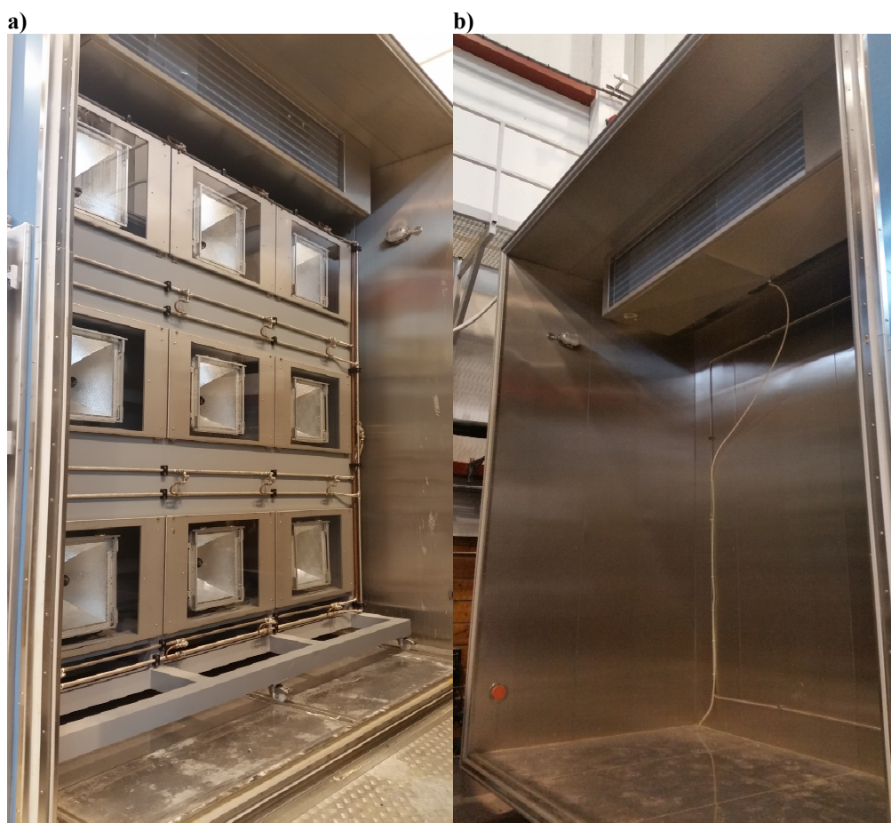
Fig. 16 Climate simulator consisting of two chambers, a) exterior side with water spray nozzles and lamps, b) interior side with space for monitoring equipment. Also showing ventilation systems at the ceilings.
