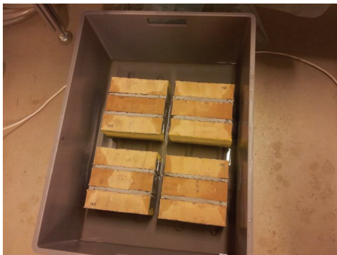
Figure 3: Absorption testing of pillar specimens, KC50-C. Tray with manually regulated water level.
