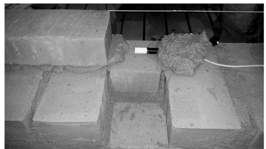
Fig. 4. Placement of Sahlen sensor in segment 5.
