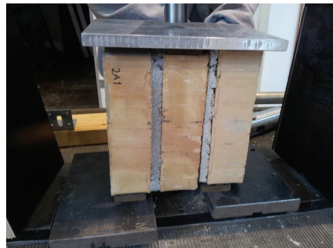
Figure 5: Shear testing of pillar specimen KC35-C. Failure in top interface of lower joint.
