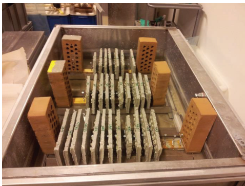
Figure 4: Absorption testing of joint specimens. Tray with automatic water level regulation.
