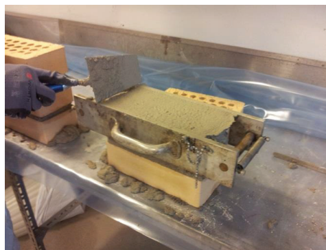
Figure 2: The brick laying and the tool used to ensure constant joint thickness.
