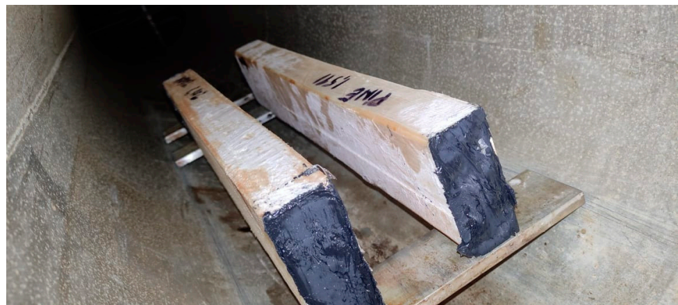
Figure 1. Specimens in the drying chamber. The white layer on the surfaces is ice due to the water thawing.
