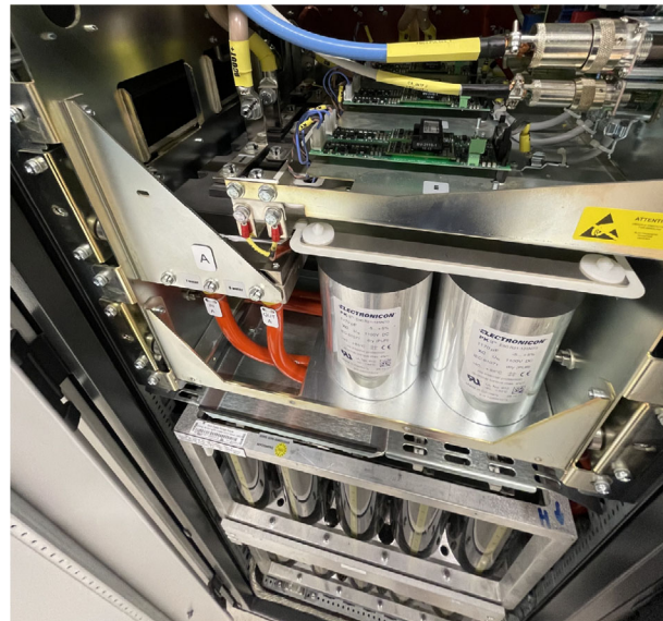
FIGURE 10 Photograph of the laboratory setup, showing the power stack, gate drivers and DC-bus filter capacitors integrated into the cabinet. The storage capacitors can be seen at the bottom.
