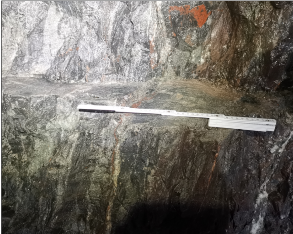
Figure 8.9: Example of the sub-horizontal joint set J3 in the amphibolite, picture taken at the same location as in figure 8.8. Strike/dip is 030/10W. Folding ruler for scale, 0.4 m.
