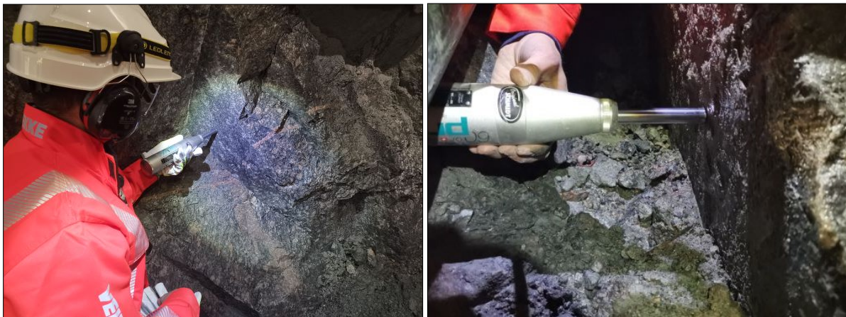
(a) JCS testing on a joint surface in the augen gneiss. (b) JCS testing on a joint surface in the amphibolite.
