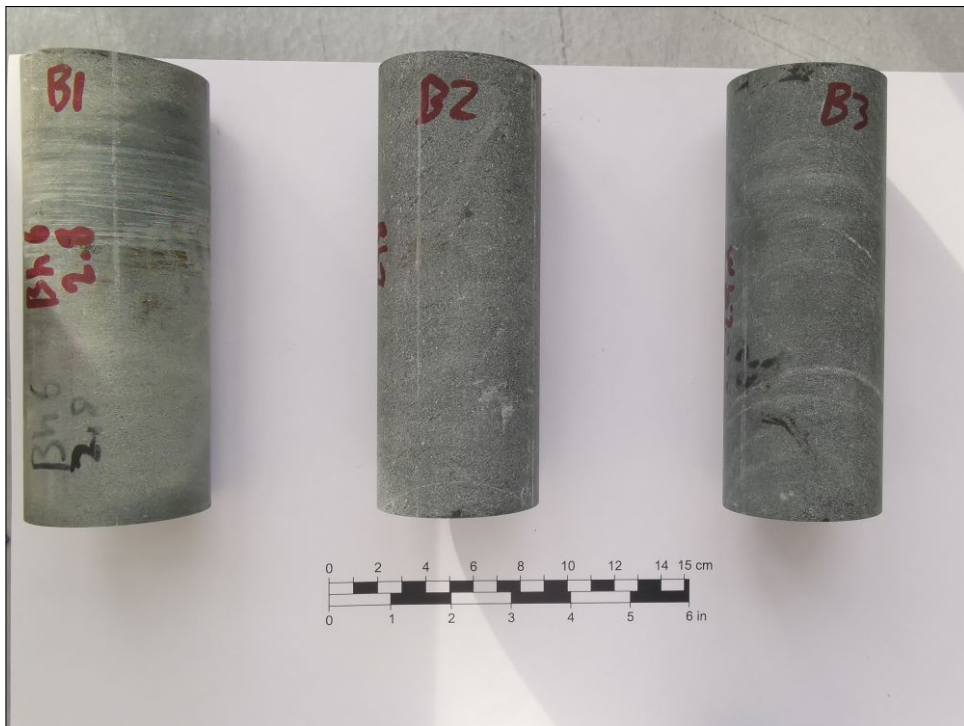
Figure 9.3: Prepared amphibolite cores, labeled B1, B2 and B3.
