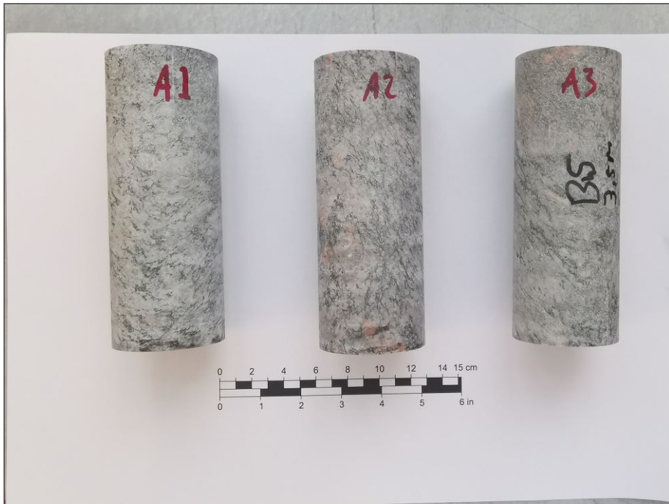
Figure 9.2: Prepared gneiss cores, labeled A1, A2 and A3.
