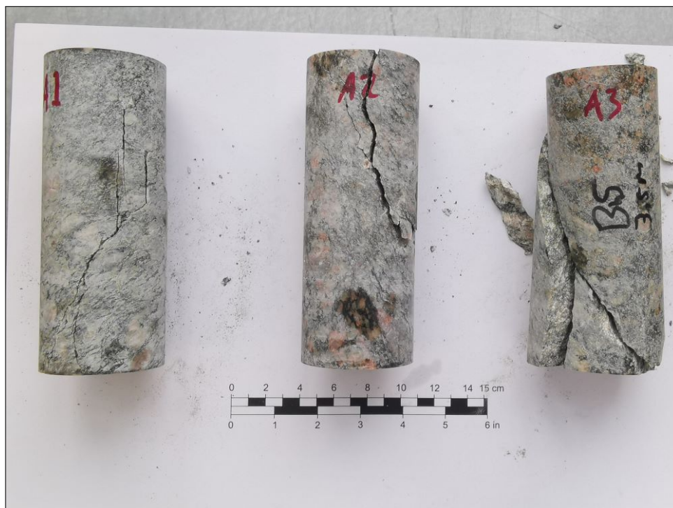
Figure 10.7: Yielded cores in the gneiss after UCS-testing.
