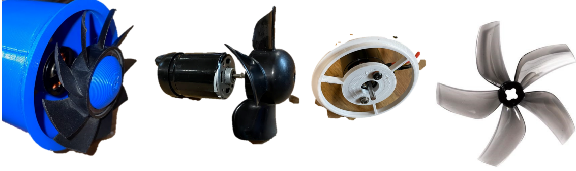
Figure 17: Different motors with some of the different fan configurations tried. The fanblade on the right is a drone fan, and is what being used in the experiment
