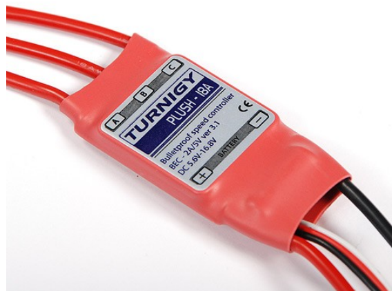
Figure 25: Electronic speed controller used. This sends 5VDC back to the arduino
