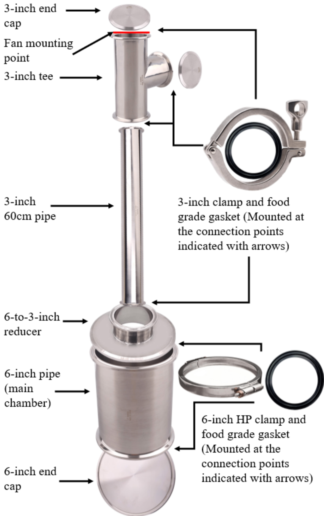
Figure 37: Overview of only the Tri-Clamp components used in the assembly
