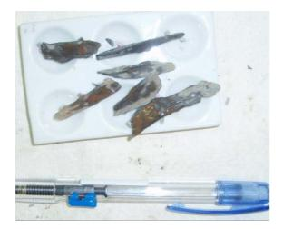
Fig. 9 Splintery cavings from breakouts in the thick shale section in the existing vertical well
