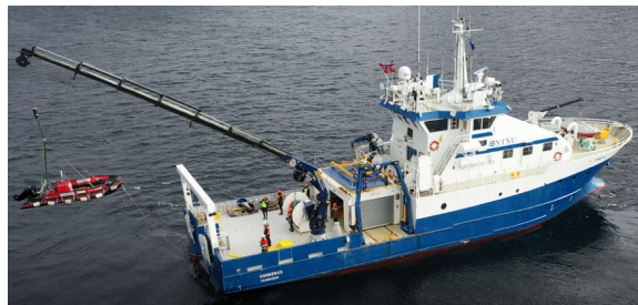
Fig. 1: A snapshot of an example operation. Excessive ship motion leads to damaging onboard equipment and compromising the safety of personnel.
