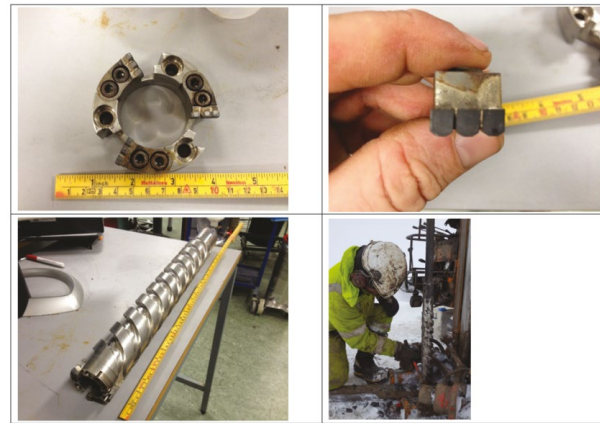
Fig. 2 SINTEF-modified CRREL coring auger (Gilbert et al., 2019)
