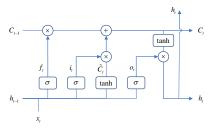
Fig. 2: The structure of the LSTM.
