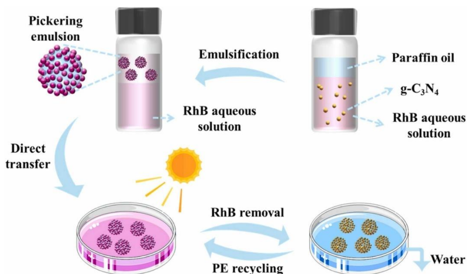
Fig. 11. Schematic of coupling process of adsorption, extraction, and photocatalysis. Reprinted from 111 with permission from Elsevier.
