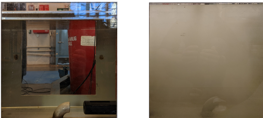
Figure 5.11: Window at the end of the first channel section (4.25 m downstream the channel inlet) during silent conditions and low flow (left) and sonication using 20 kHz ultrasound, leading to the creation of a micro-bubble cloud, and high flow (right).
