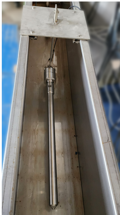
Figure 5.5: SinpaTec 20 kHz rod transducer used during degasification experiments in the medium-sized test rig (seen from the top), installed in the first section of the channel.
