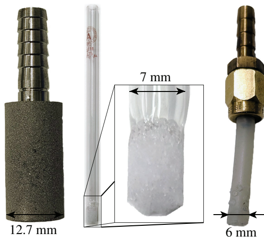
Figure 4.9: Gas diffusers used for air bubbling in the reactor. The pore size for the oxygenation stone, the ace gas diffuser and the synthetic tube with holes is 0.5\ \mu\text{m} , 145\ \mu\text{m} to 174\ \mu\text{m} and 2\ \text{mm} , respectively. The data is available in Table A.4.
