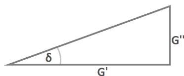
Figure 1-8 Schematic depiction of the relation of storage modulus ( G' ) to loss modulus ( G'' ) expressed by the phase angle ( \delta ).
