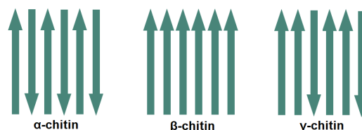
Figure 1-29 Illustration of the poly-N-acetylglucosamine chain arrangement within the three different crystalline forms of chitin, \alpha -, \beta - and \gamma -chitin
