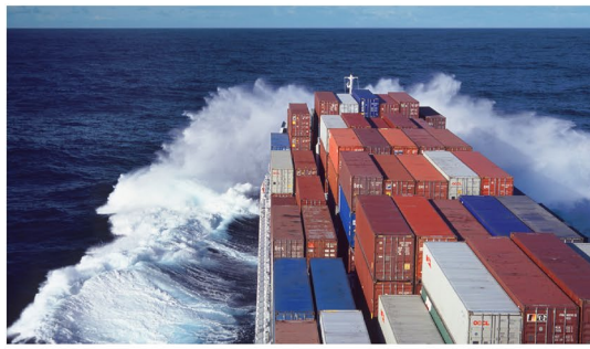
(a) Photo from the bridge of the considered vessel; a 2800 TEU Panamax container ship.
