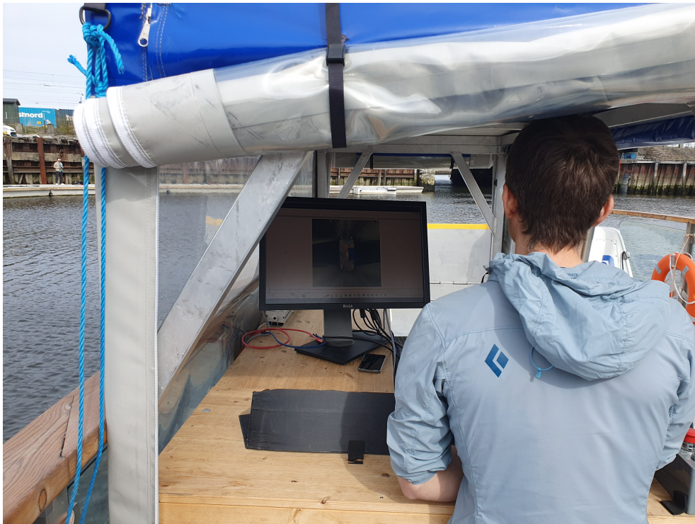
Figure 6.5: An image of how the operator (to the right) was able to see the IPM image on a monitor (to the left) while operating the ferry towards the dock in front.
