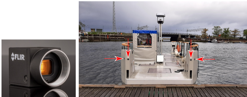
(a) An image of the FLIR Blackfly S 50-S5C camera used on milliAmpere2. Image courtesy of Edmund Optics, Inc [27]. (b) An image of milliAmpere2 with red arrows pointing at 4 of the camera positions. Photo taken from the thesis proposition web page, hosted by AUTOFERRY [28].
