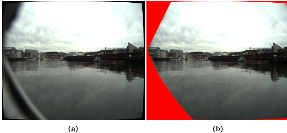
Figure 4.5: Showing an arbitrary image from camera fs_f . In a) the hull surrounding the camera is visible on the left side. The mask to remove the hull from the IPM image is the area covered by red in b).
