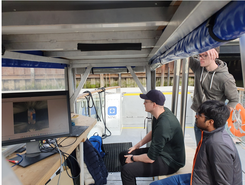
Figure 7.5: An image showing the operator's view during docking. Clearly, it is difficult to observe the dock behind the ramp. However, on the bottom part of the monitor on the left-hand side of the image, the dock can be observed by the operator in the bird's eye view image.
