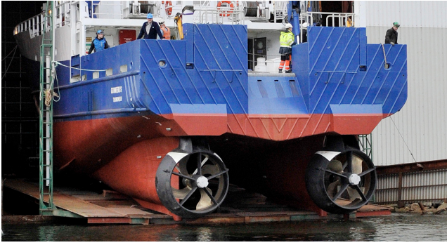
Fig. 2. RV Gunnerus in dock showing the two stern rim-driven azimuth thrusters. Courtesy of Kongsberg Maritime AS
