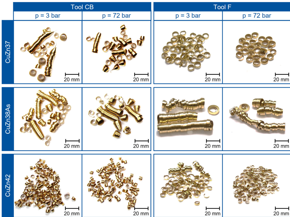
Fig. 9 Overview of chips produced in the cutting of the three workpiece materials at f = 0.15 mm/r
