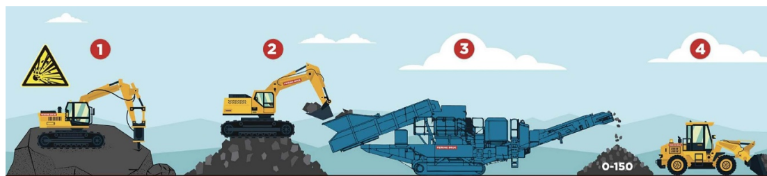
Figure 6. Steps included in crushing plant stage 1 (Feiring Bruk 2018a). Reproduced with permission from Feiring Bruk AS.
