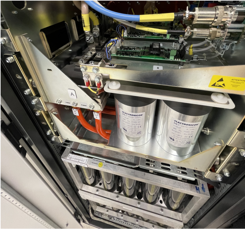
Figure 4.13: Photograph of the laboratory set-up, showing the power stack, gate drivers and DC-bus filter capacitors integrated into the cabinet. The storage capacitors can be seen in the bottom.
