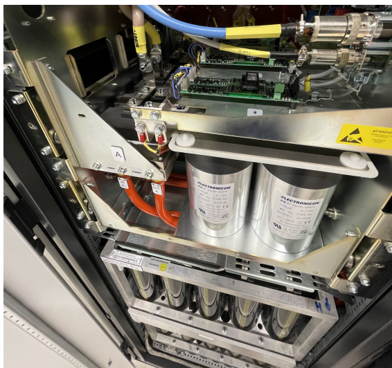
Figure 4.23: Photograph of the laboratory set-up, showing the power stack, gate drivers and DC-bus filter capacitors integrated into the cabinet. The storage capacitors can be seen at the bottom.
