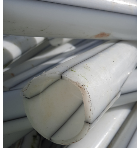
Figure 3: White feed pipe sample acquired from the recycler. The carbon black stripe is to prevent static electricity, and makes the polymer a uniform black after melting.
