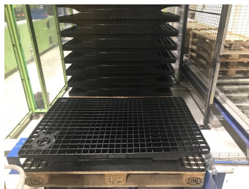
Figure 5: Walkways produced for an aquaculture fish farm.
