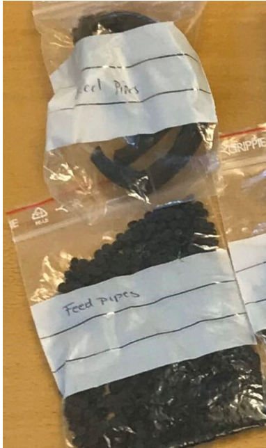
Figure 2: Two feed pipe samples acquired from the recycler. The top one is washed and coarsely ground, while the bottom have been melted into pellets.
