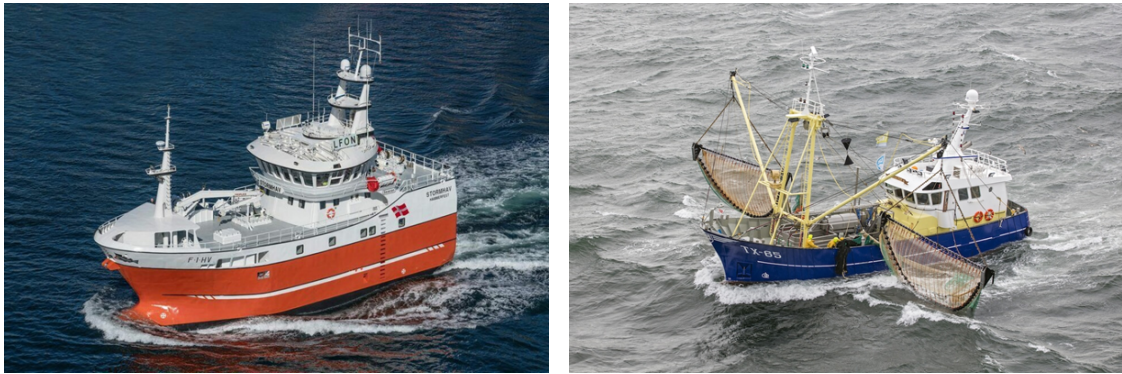
(a) The 27.99 metres long conventional coastal vessel MS Stormhav (Skipsrevyen, 2020). Foto: JK Foto (b) The 23.95 metres long shrimp trawler Bona Fide (Maritime, 2018)
