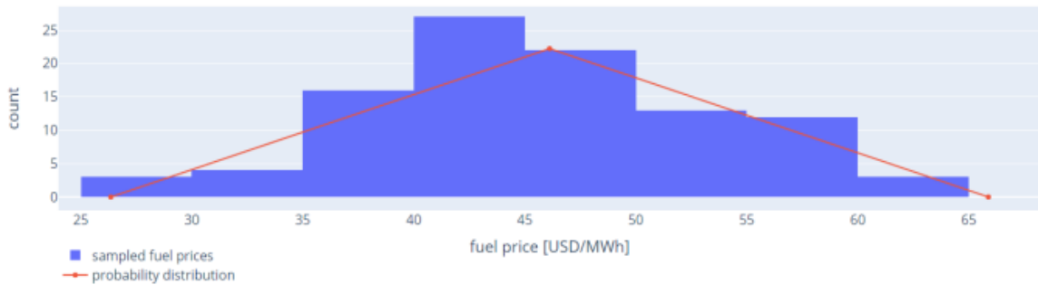
Figure 6.2: Sampled and discounted fuel prices for VLSFO in period 1, set with 100 scenarios (Lagemann et al. 2023a)
