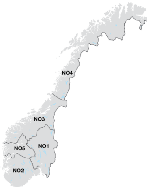
Figure 2.13: This map show the five electricity price bidding areas in Norway (Statnett, 2022).
