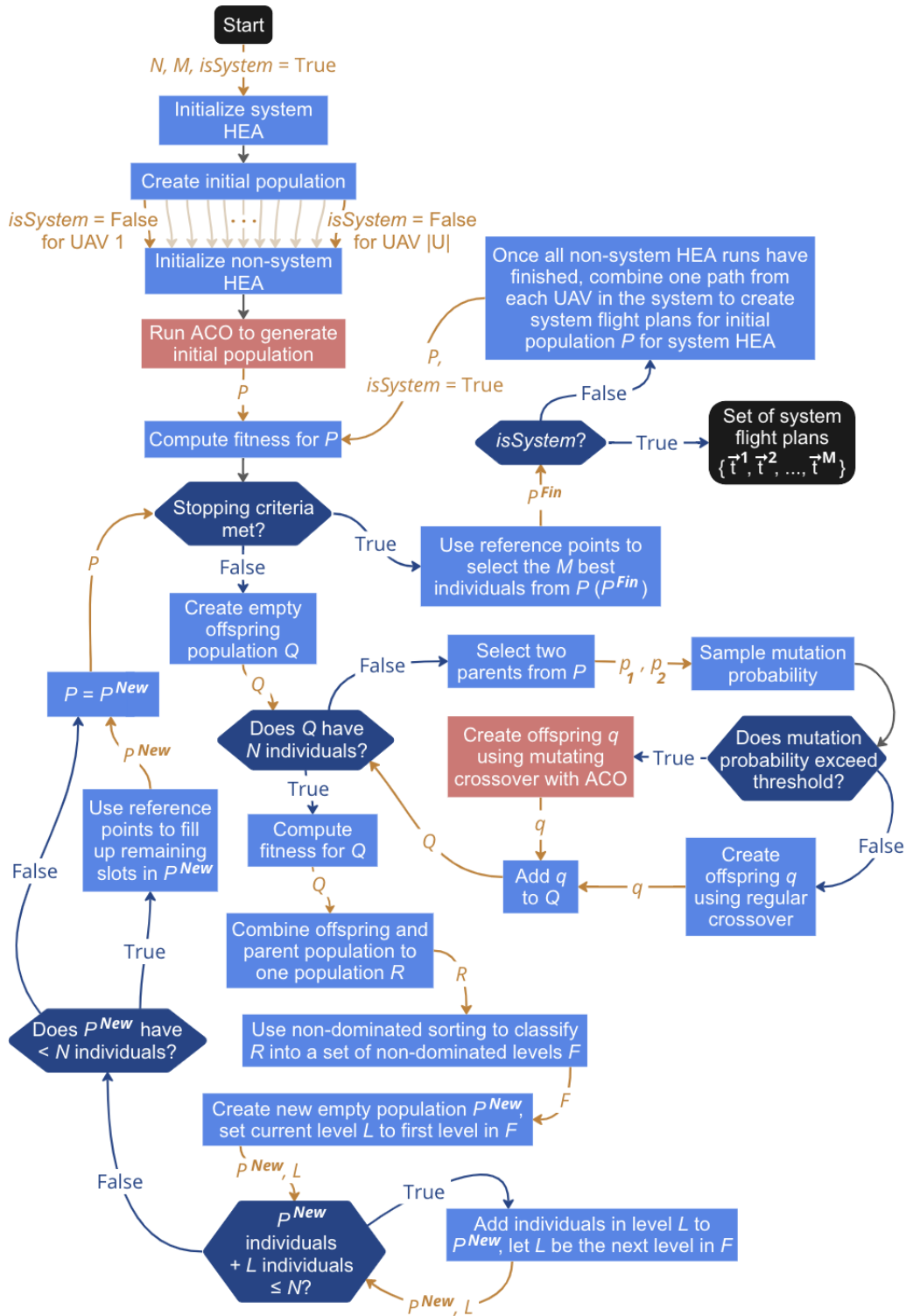
Figure 7.1: A flowchart for the hybrid evolutionary algorithm (HEA) for a system of UAVs. Blue boxes are steps in the NSGA-III base, while dark blue hexagons are if-statements with corresponding dark blue result arrows. The light red boxes are steps using ACO. The two black, rounded boxes correspond to the start and end points of the algorithm. Orange arrows means the value on the arrow was created or updated by the box the arrow originates from.
