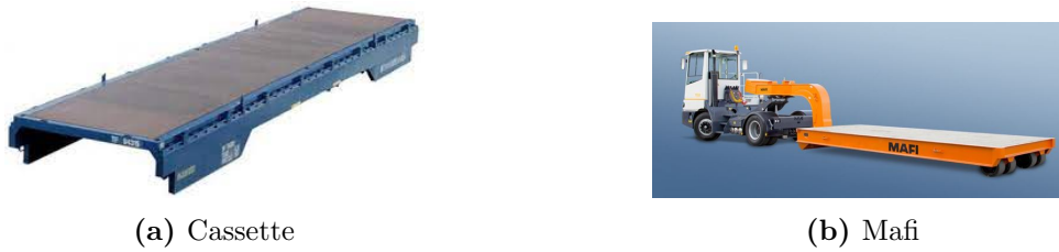
Figure 2.8: Load carriers types used to transport goods with ro-ro vessels in Hydro's new maritime logistics network
