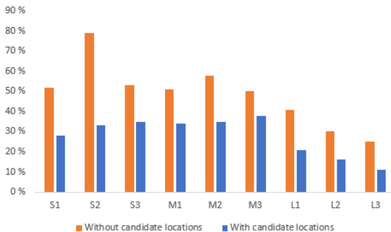
Figure 8.2: The average extra travel time for drivers in each instance group with ridesharing
