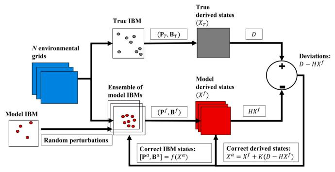
Fig. 1. A conceptualization of the assimilation of data using the twin model experiment.
