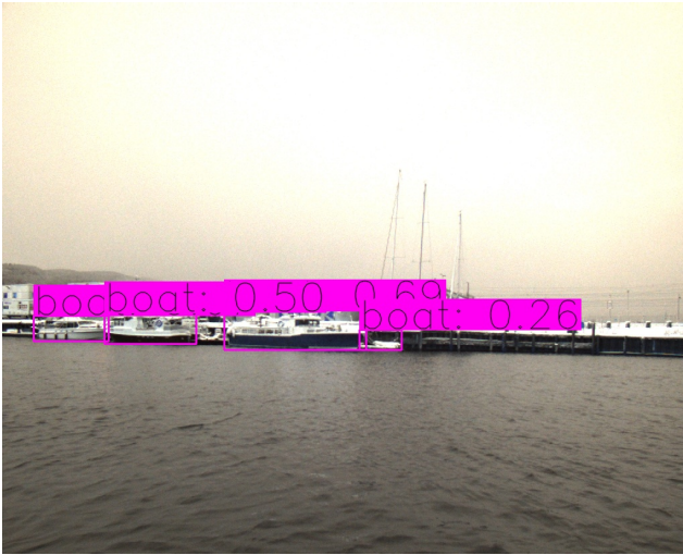
Figure 3: Detection output from the Yolo v4 on an image from the experimental validation in the Canal in Trondheim. The algorithm detects four leisure boats docked along the Canal.
