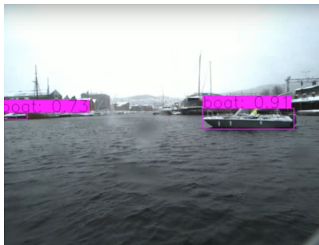
Figure 9: Crossing 3, target intersecting ownship trajectory, inducing COLAV maneuver.
