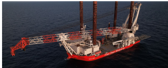
Figure 26: Bold Tern jack-up vessel with the upgraded crane (Fred. Olsen Windcarrier, 2022)
