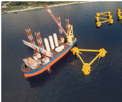
Figure 14: Concept art of a jack-up vessel used for the floating wind turbine integration (Associated British Ports, 2023)
