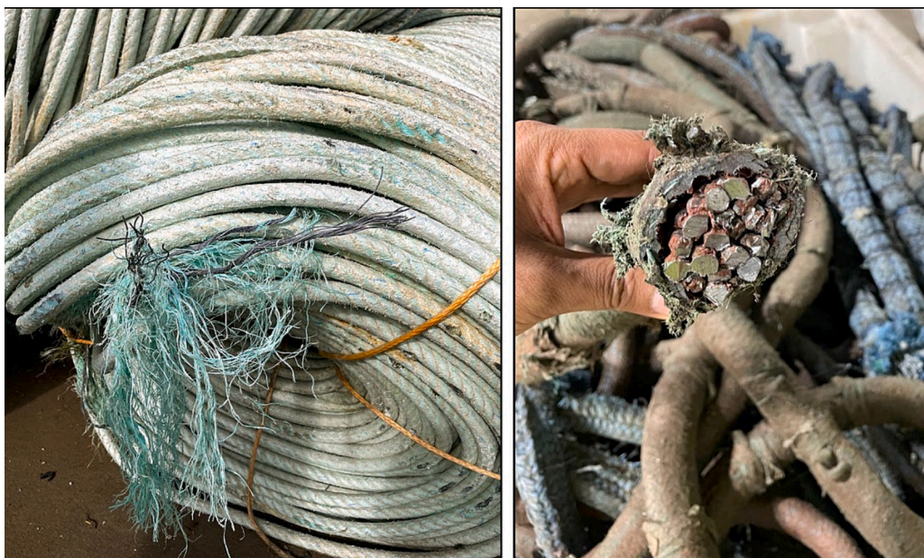
Fig. 7. End-of-life ropes with a) steel wire and b) lead as a core.
