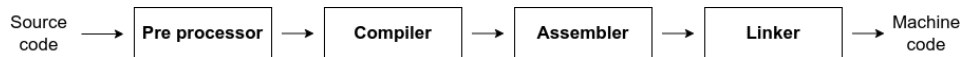
Figure 1: The steps a C compiler goes through transform source code to machine code.
