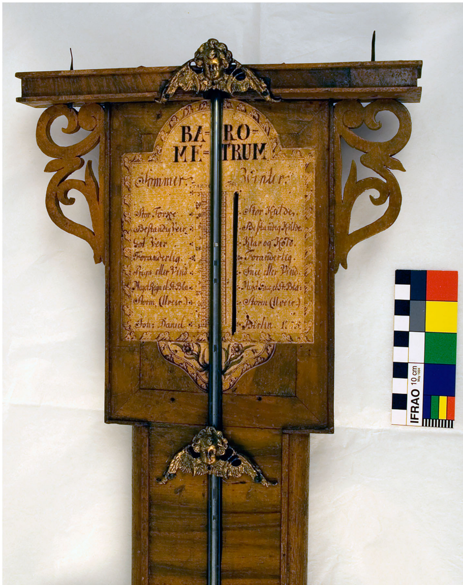
Figure 4. Johan Daniel Berlin's barometer, with measurement scale for summer, on the left side, and scale for winter, on the right. Image by Ivonne Geisler, NTNU University Museum.
