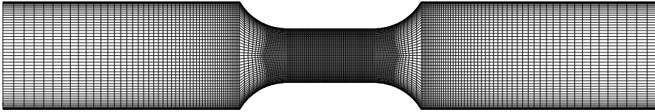
Figure 7.17: FE mesh of the full smooth tensile specimen.
