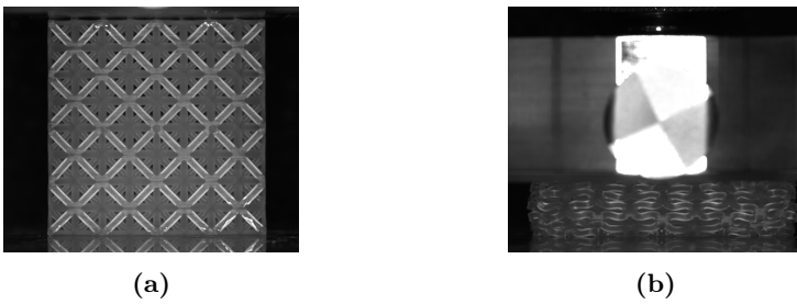
Figure 4.8: Images captured by the digital camera from a compression test with v = 3 mm/min from (a) before the test started and (b) at the point of maximum cross-head displacement.
