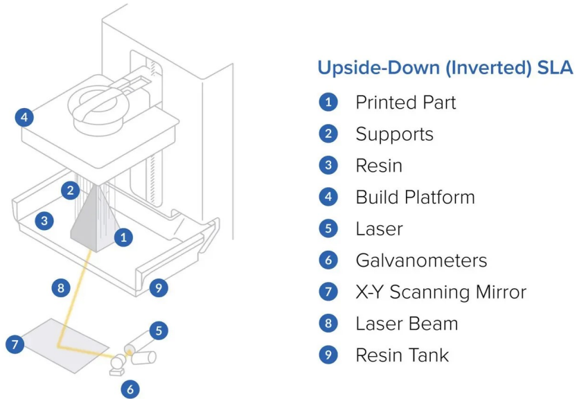
Figure 1.1: A graphical representation of the principles of SLA 3D printing [5].
