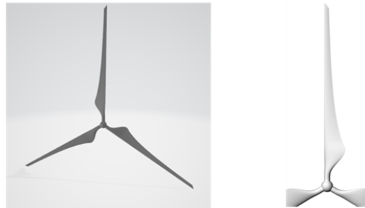
Figure 3. CAD model of the performance matched model-scale blade design perspective (left) and front view (right).
