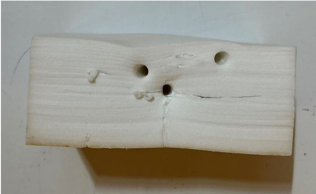
Figure 3.2.1: RS sponge after the vacuum freezing, with visible locations of measurements
