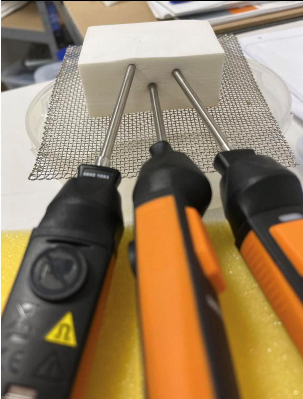
Figure 3.2.2: RS sponge with temperature sensors before the vacuum freezing process
