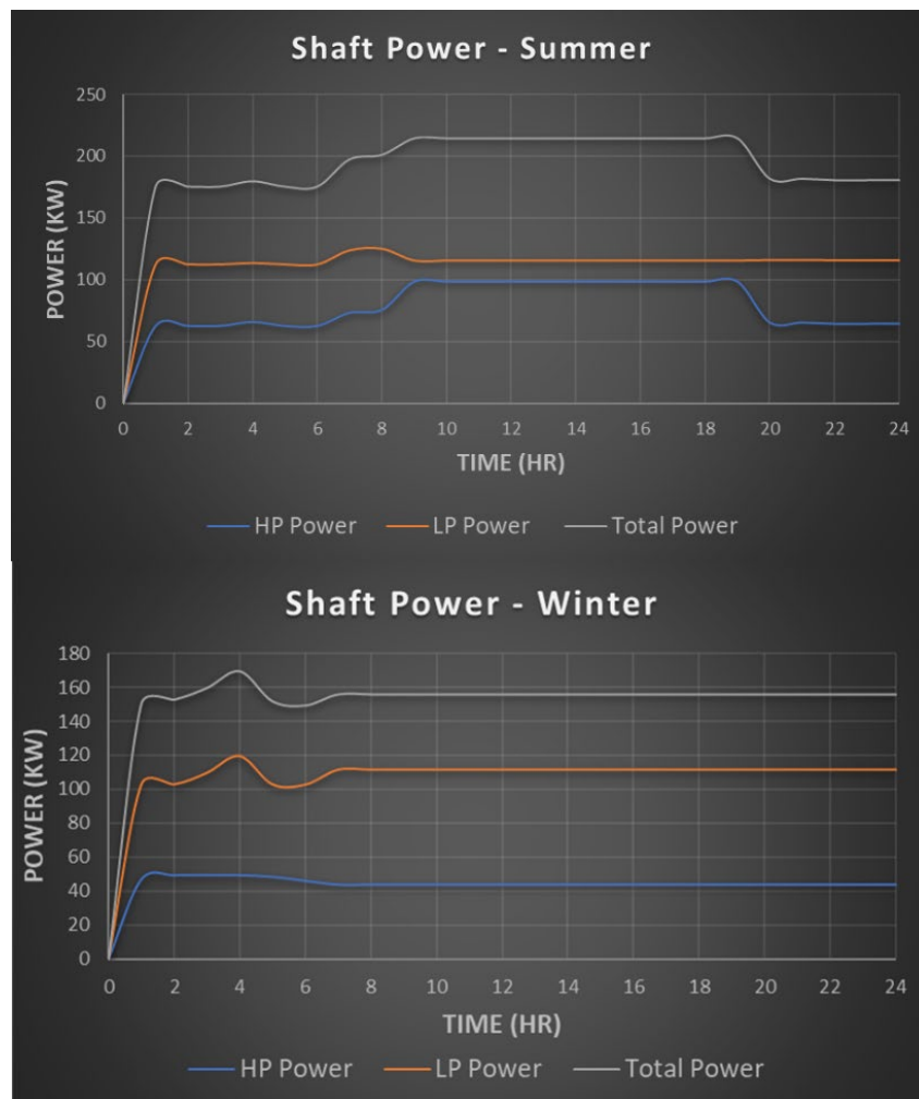
Figure 48: Temporal variation of shaft power for individual separators and total system across seasons
