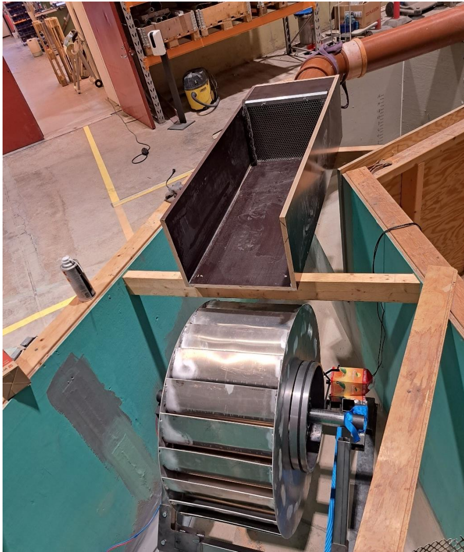
Figure 8 - Channel and hydropower unit installed in the hydrotechnical laboratory. The original channel's length denoted as "-15", since it was easier to add length extensions than to shorten the channel.
