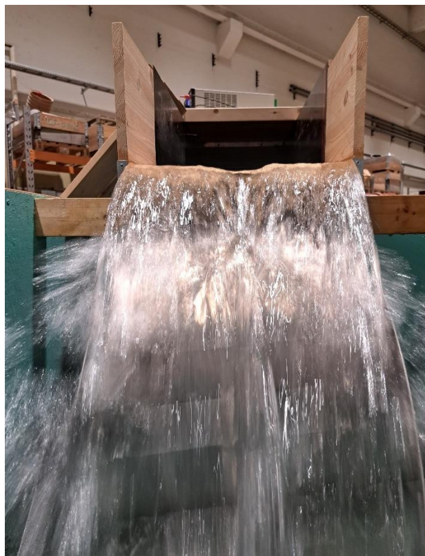
Figure 38 - Picture from one of the videos showing the splashes that were almost always present in higher discharges and rotation speeds.
