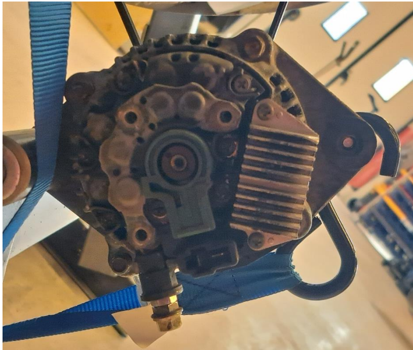
Figure 39 - Detailed photo of the diode bridge rectifier of the alternator used in the experimental prototype unit.
