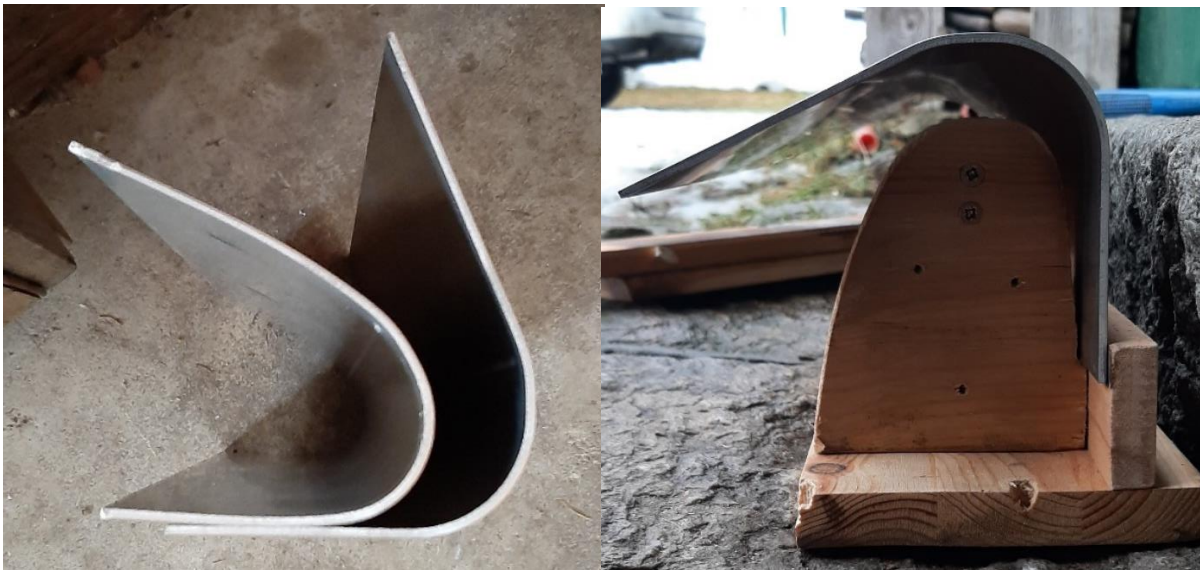
Figure 33 - Comparison of the provided and final shape of the buckets (on the left), and the wooden form used to bend the heated semi-finished buckets (on the right).
