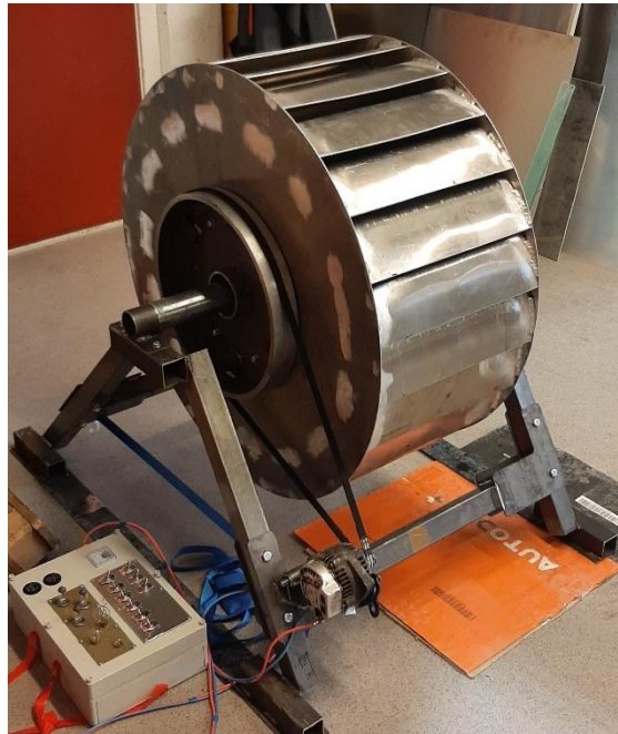
Figure 7 – Left side of the prototype with visible pulley system transferring the rotation to the car alternator. First “lightbulb” version of the Load box can be seen in the bottom left corner of the picture.
