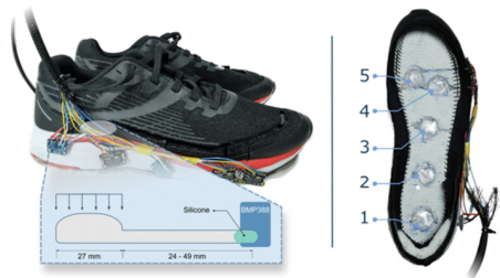
Fig. 1. Left: illustration of the sensor geometry and the shoe prototype used in this study. Right: the layout of the sensor array in each sole. In use, the array is covered by the insole.
