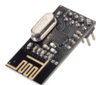
Fig. 1. An RF communications module identical to those used in this case report, based on the nRF24L01+ transceiver. Manufactured by Seeed Studio.
