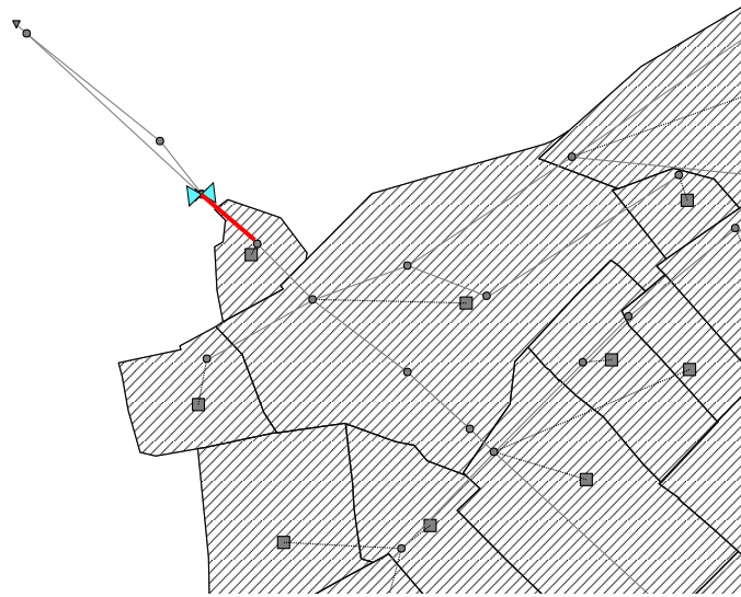
Figure 10: Pipe L190252 (red) leading into OF07 (blue) was used in the calculation of the volume reduction entering the system caused by BRC. Zoomed in figure from the SWMM model map.
