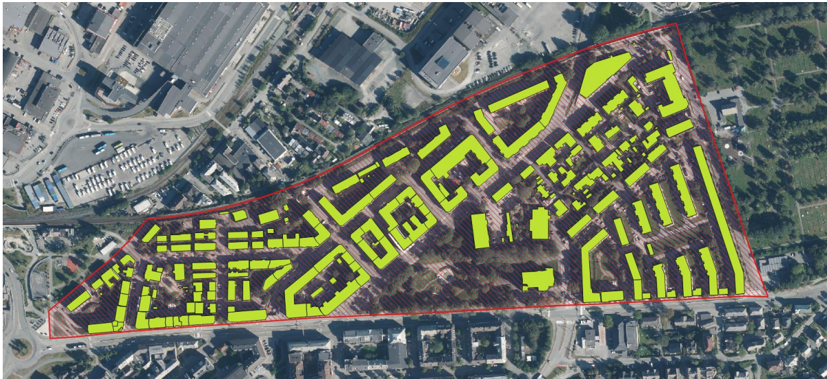
Figure 8: Project area (marked red) and roof area (marked green) as polygons (shapefile) in QGIS.
