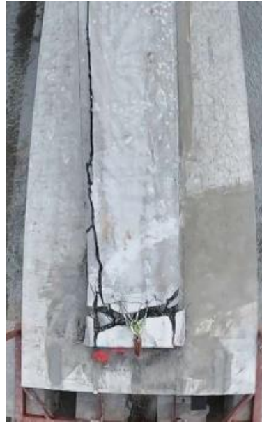
f) The end of impactor after the first impact
