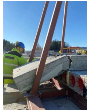
b) Tensile damage at floor slab after the second impact
