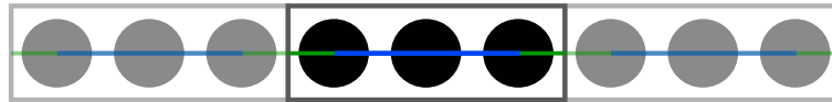
Figure 3.2: In this figure the length is measured as a "center of outer atom" to "center of outer atom on opposing side" represented by the blue line. The green lines represent "half the bond length" and by adding them we now have the length of the repeating structure.
