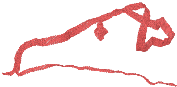
Figure 3.3: Hydrogen-free GNR that curls up and reacts with itself during the equilibration steps of AEMD simulation.
