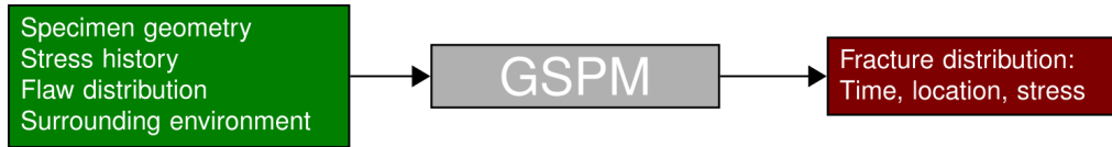
Figure 3.1: The overall inputs and outputs of the GSPM. The model needs information about the specimen geometry, stress history, flaw distribution and the surrounding environment, and predicts the fracture distribution in terms of fracture time, location and stress.
