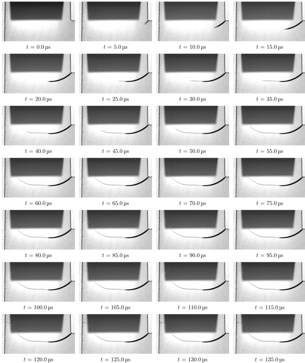
Figure 4.8: Time-lapse of crack propagation for one of the experiments. The upper dark gray field is the shadow of the testing machine.
