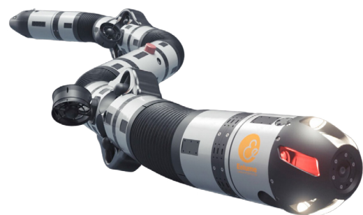
Fig. 1. The Eelume AIAUV, a highly redundant UVMS
