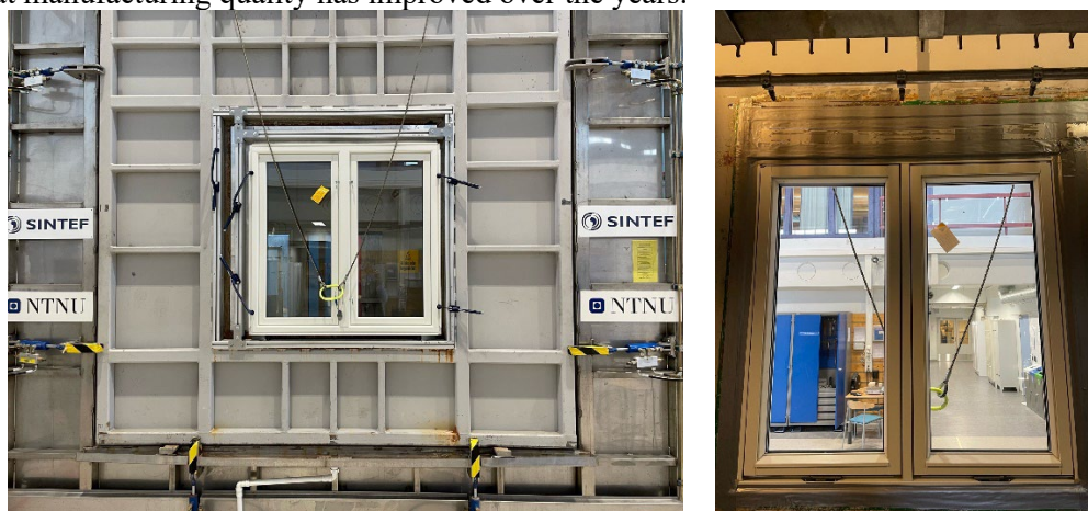
Figure 2: Window specimen mounted in test chamber. Left: Window interior side. Right: exterior.
