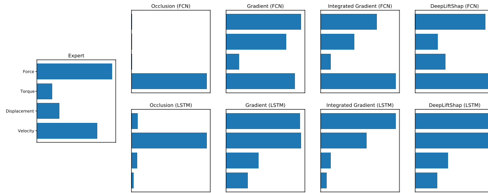
Fig. 6: Relevance score provided by the expert and the global sensor attribution calculated from different XAI methods for the medical device assembly
